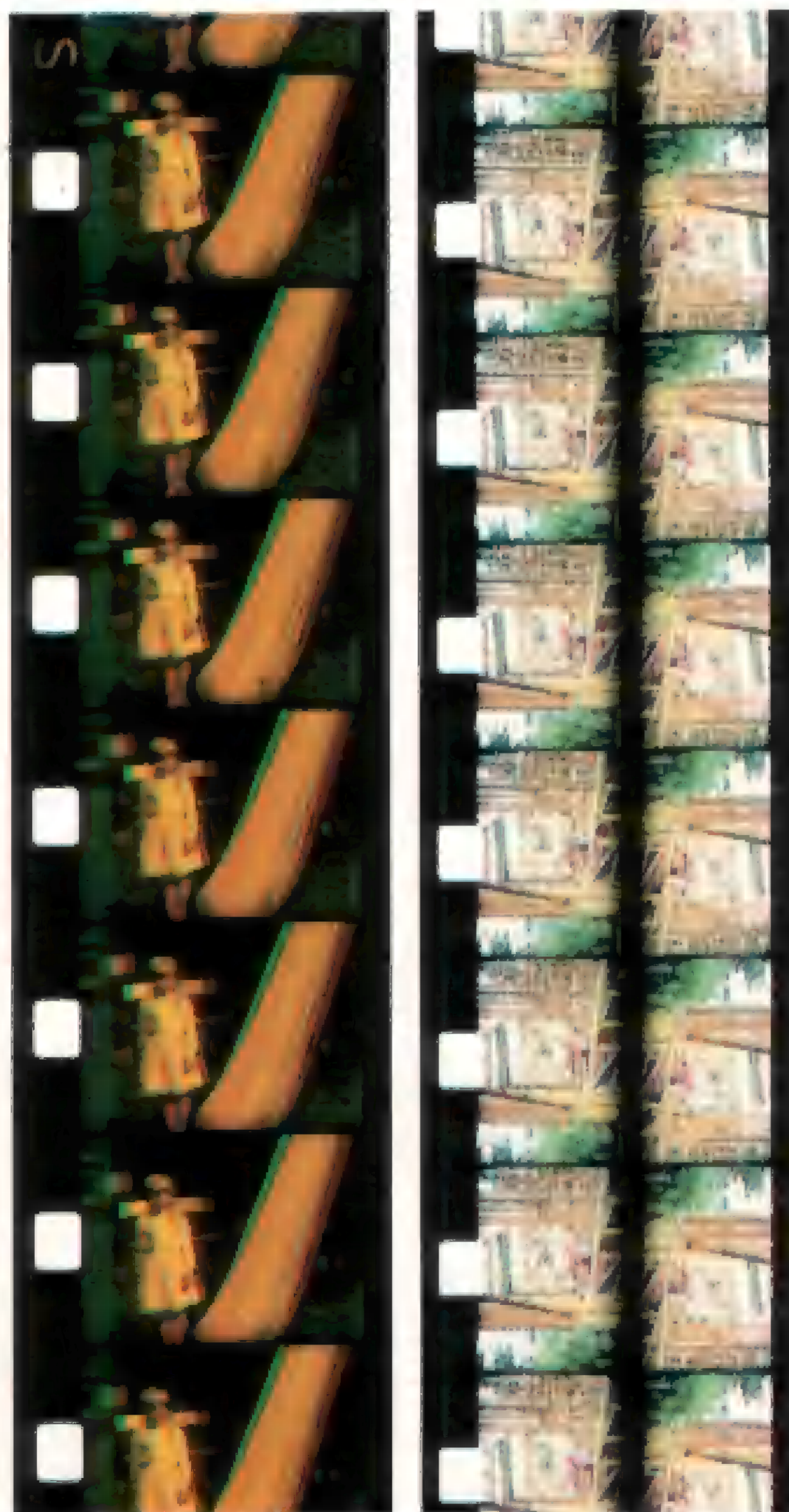
Opposite top: The Spondon 3-D attachment. Above: Bolex 3-D positions the left and right images side by side. Below left: Spondon 3-D creates a red/green anaglyph 3-D image using the entire Super-8 frame. Below right: Widescreen 3-D Super-8 is possible with attachments that split the frame and rotate the image.
